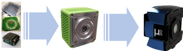
DM development: achieved R&D steps during the DynAMic project, from components and sub-assemblies (left), to first prototypes (middle), and final product (right)
